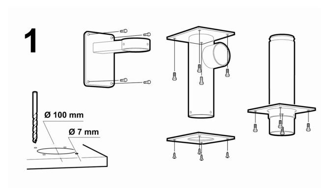
1.) Install mounting brackets. Table mounting: Drill holes.
