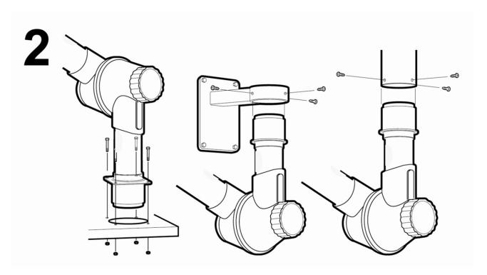
2.) Fit the arm to bracket. Table mounting: Fit arm in hole.
