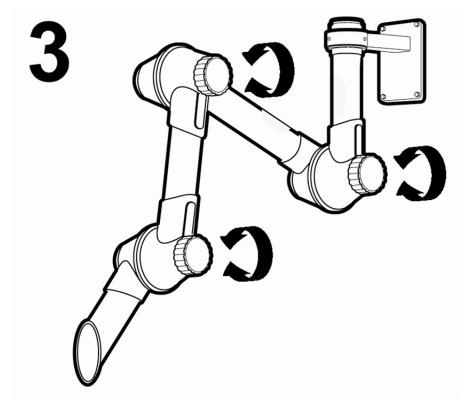
3.) Adjust the tension in the plastic joints. Check that the adjusting knobs are placed to the right.
